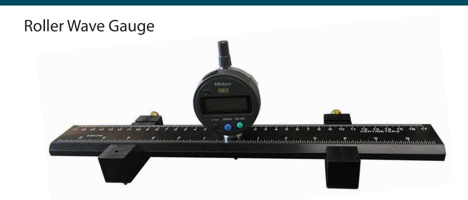
Roller-wave gauges are used for measuring roller wave in accordance with ASTM Test Method C1651, Glass Association of North America (GANA), and other accepted test methods. Measured peak-to-valley depth and wave length values are used to calculate optical distortion using a simple equation or supplied Excel software. Strainoptics offers four high-quality roller-wave models with flat-bottom or three-point contact surfaces.
