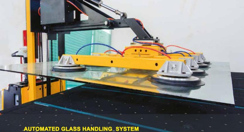
With a maximum load capacity of over 600 kilograms, our vacuum lifter can handle glass size of up to 2440 X 3660 mm. Our vacuum lifter can also move laterally for easy handling and can turn in its own radius, which means tighter but smoother turning point. Electronic assistant tilting ensure that maximumcare is taken for glass transportation.
